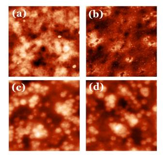
Figure 4. Atomic Force Microscopy (AFM) of dried films formed from a binary mixture of large particles and small pH-responsive particles, with number ratio of N<sub>L</sub>:N<sub>S</sub> = 1:800 and an initial solids content of 10 wt%. Height images (5 x 5  $\mu$ m<sup>2)</sup> obtained from for four different pH values of the initial dispersion: (a) pH 3, (b) pH 4, (c) pH 7 and (d) pH 9.5.
