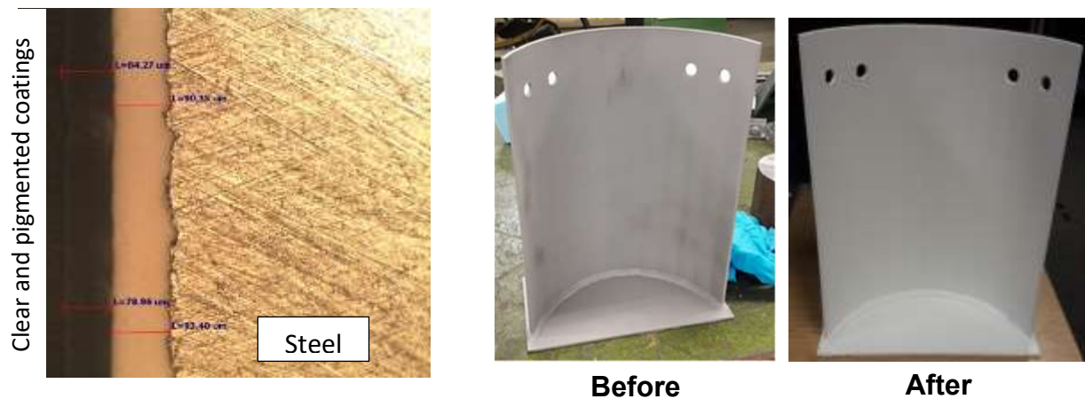
Fig. 8. An optical micrograph of the cross-section of a clear topcoat on a pigmented base coat on a blasted steel panel (at left). A miniature steel structure is shown before and after the spray application of a pigmented coating (at right).
