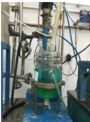
Fig. 7. Glass reactor used for scaling up of the surfactant-free latexes
