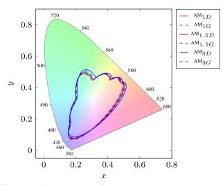
Fig. 10. Influence of the illumination on the perceived color  $(Si_3N_4 ARC)$  at normal incidence for different irradiances.
