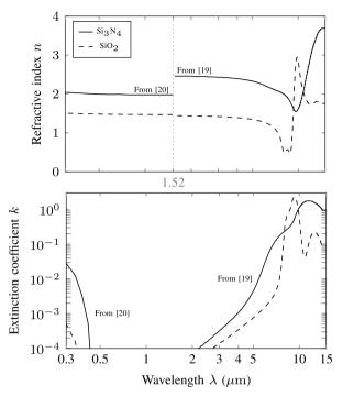
Fig. 5. Refractive index of  $SiO_2$  and  $Si_3N_4$  to cover both the visible and long wavelength infrared domains (data extracted from [18-20]).
