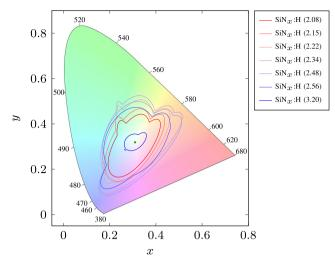
Fig. 20. CIE1931 color space chromaticity for different  $SiN_x$ :H ARC layers with an  $AM_{1.5G}$  irradiance (optical index at  $\lambda = 600$  nm in brackets) when taking the EVA and glass layers into account. The green point in the center of the gamut corresponds the simulation with no ARC.
