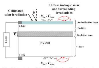
Fig. 3. Description of the simulated solar cell and its boundary conditions.
