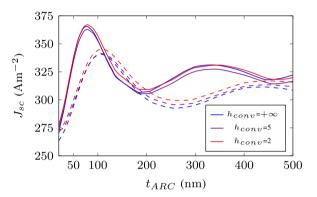
Fig. 17. Short current circuit current density as a function of the ARC thickness (solid lines:  $Si_3N_4$ , dashed lines:  $SiO_2$ ).
