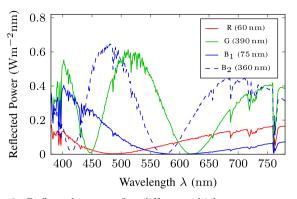
Fig. 9. Reflected power for different thicknesses at normal incidence.
