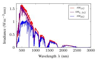
Fig. 4. Spectral irradiances for different air masses.
