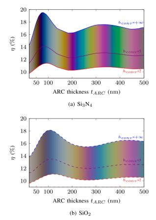
Fig. 19. Conversion efficiency and perceived color for different single layer ARC thicknesses (with  $\theta = 0$ ).
