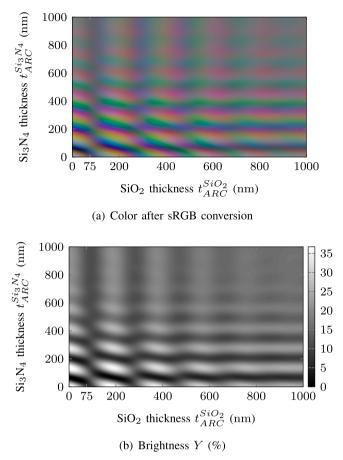
Fig. 12. Perceived color and brightness converted into sRGB for a  $SiO_2/Si_3N_4$  double layer ARC at normal incidence.
