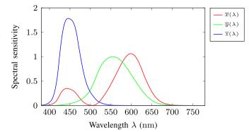
Fig. 1. CIE 1931 standard observer color matching functions.
