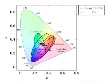
Fig. 8. CIE1931 color space chromaticity for a Si<sub>3</sub>N<sub>4</sub> ARC with an AM<sub>1.5G</sub> irradiance. For  $\theta = 0$ , arrows represent the direction for which  $t_{ARC}$  is increasing and round marks correspond to ARC thicknesses multiples of 25 nm.
