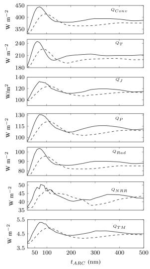
Fig. 15. Heat and sink sources as a function of the ARC thickness (Solid lines:  $Si_3N_4$ , dashed lines:  $SiO_2$ ).
