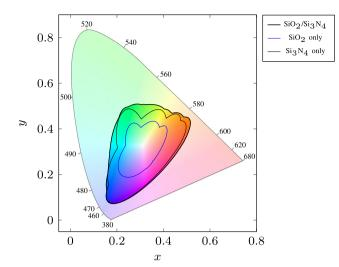
Fig. 13. CIE xyY 1931 color space for a double-stack ARC layer  $(\rm SiO_2/Si_3N_4)$  with an  $\rm AM_{1.5G}$  irradiance.
