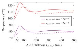
**Fig. 14.** Solar cell temperature as a function of the ARC thickness under  $AM_{1.5G}$  illumination. For  $h_{conv} = +\infty$ , temperature is 25 °C whatever  $t_{ARC}$ . Solid lines: Si<sub>3</sub>N<sub>4</sub>, dashed lines: SiO<sub>2</sub>.
