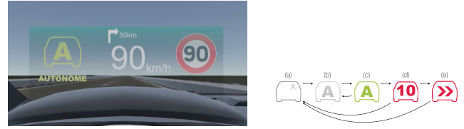
Figure 1: The HUD of the target vehicle and the symbols that represent the states of the vehicle: (a) manual driving, (b) autonomous driving system available (c) autonomous driving system activated, (d) take over request with countdown, (e) emergency brake. The arrows represent the possible transition between the states.
