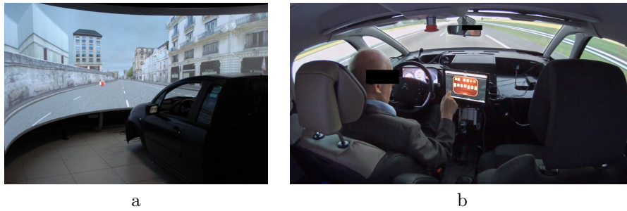
Figure 4: The test drive simulator: (a) the real cabin with the 170 degree panoramic display and (b) a view of the cabin interior
