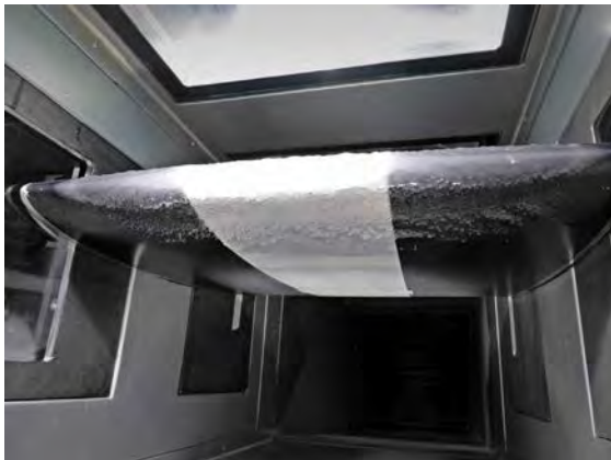
Fig. 9. NACA 0012 airfoil covered with ice layer inside the IWT test section.
