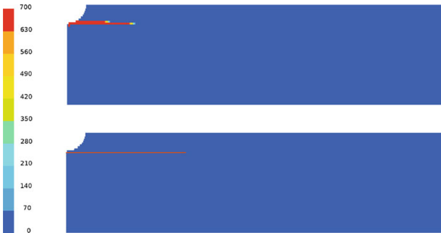
Fig. 23.19 Simulation of a [0_2/90_2]_S tension test: computed microcracking density maps closed to final fracture (with and without splits)
