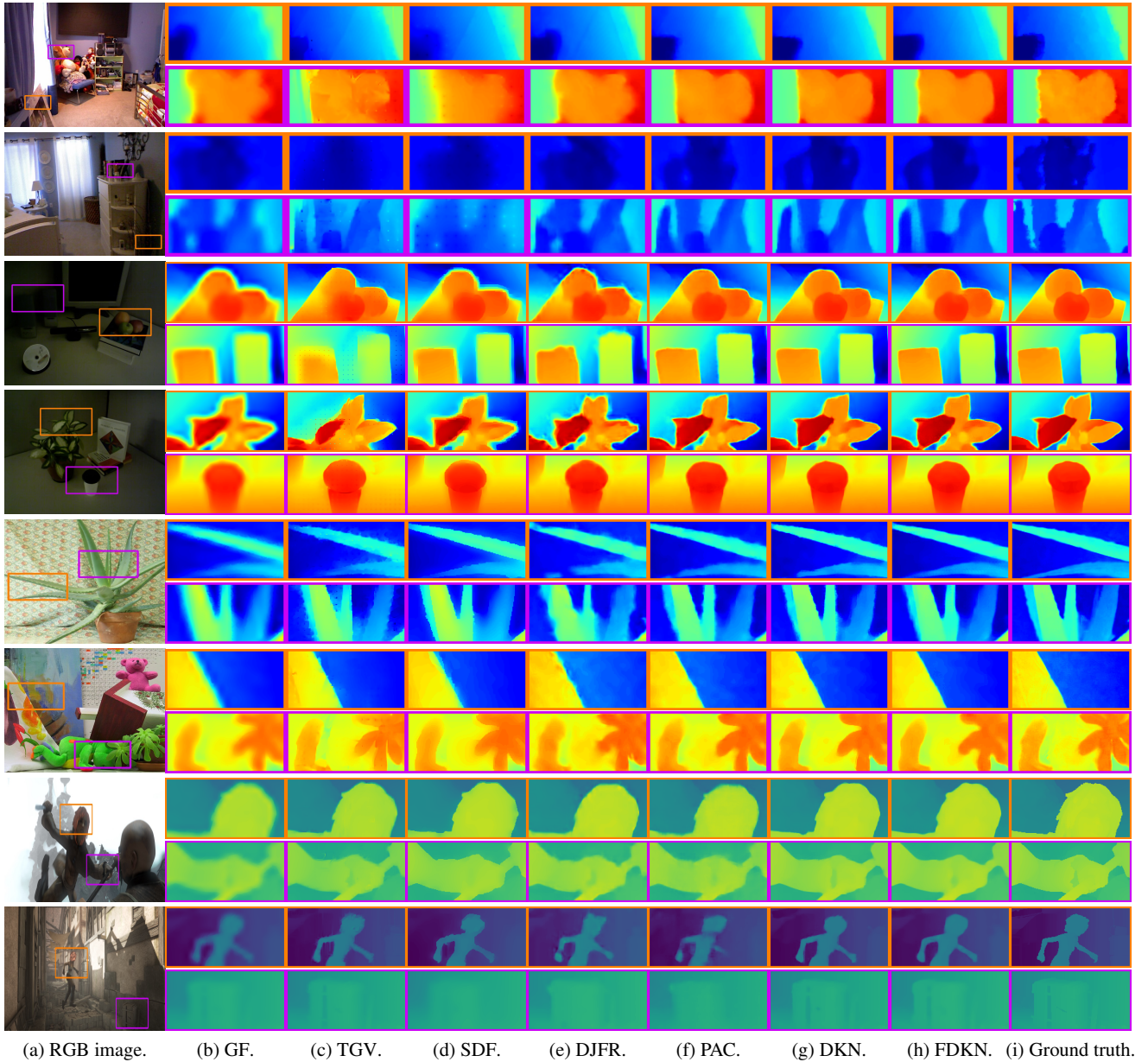
Fig. 6 Visual comparison of upsampled depth images ( 8\times ): (a) a RGB image, (b) GF (He et al. 2013), (c) TGV (Ferstl et al. 2013), (d) SDF (Ham et al. 2018), (e) DJFR (Li et al. 2019), (f) PAC (Su et al. 2019), (g) DKN, (h) FDKN, and (i) ground truth. Top to bottom: Each two rows show upsampled images on the NYU v2 (Silberman et al. 2012), Lu (Lu et al. 2014), Middlebury (Hirschmuller and Scharstein 2007) and Sintel (Butler et al. 2012) datasets, respectively. Note that we train our models with the NYU v2 dataset, and do not fine-tune them to other datasets.
