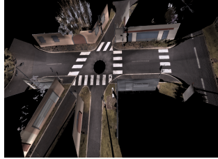
(d) Outdoor point cloud after sampling containing 2 732 783 points
