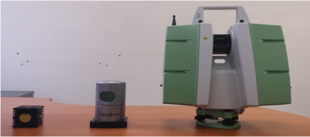
Figure 14: Sensors used to test the CICP approach. From left to right: SR4000 Time-of-Flight camera, Velodyne HDL 32-E, and Leica P20 Laser.
