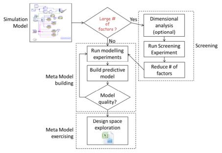
Figure 11: Meta model synthesis process
