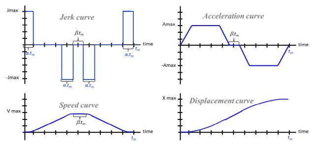
Figure 6: S Curve displacement for mechanical profile
