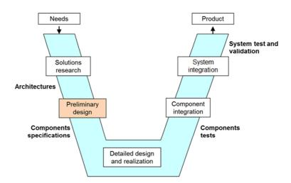
Figure 1: V-cycle design for a mechatronic system
