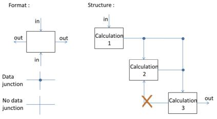
Figure 8: N<sup>2</sup> diagram principle
