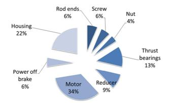
Figure 14: Mass distribution of an optimal sizing (pitch of 5 mm/rev)
