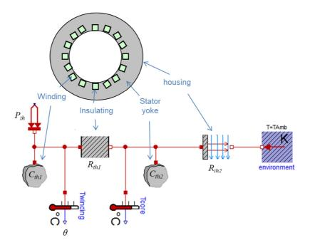
Figure 13: Thermal model of the motor
