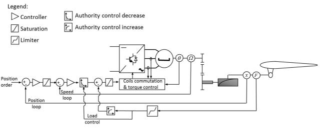
Figure 5: Control architecture
