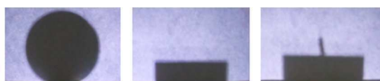
Figure 1. Shadows of a tea candle on the paper screen of the projecting box
