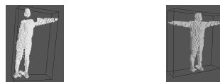
Figure 3: A depth first (left) and width first (right) octree carving with the same elapsed time. The former leads to an unbalanced space carving, the latter to a balanced one.
