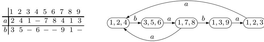
**Fig. 3.1.** An automaton of  $S$ -degree 3.
