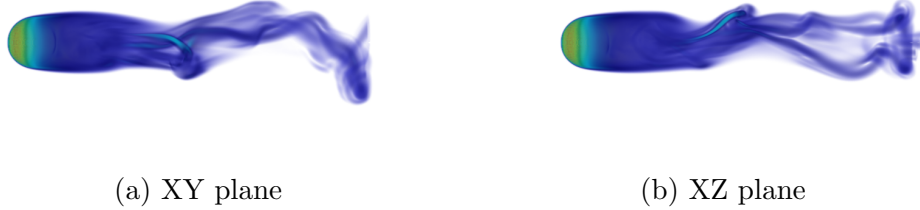
Figure 12: 3D instantaneous vorticity norm |\boldsymbol{\omega}| at T = 40 for flow past a sphere at Re = 1000 .
