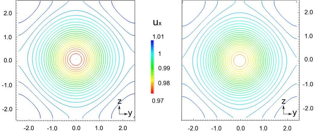
Figure 3: Flow past a 3D sphere: isocontours of the inlet streamwise velocity  $u_x$  in the YZ plane when imposing periodic boundary conditions coupled with adapted corrections. (Left picture) The width of the absorption band equals 1. (Right picture) The width of the absorption band equals 2.
