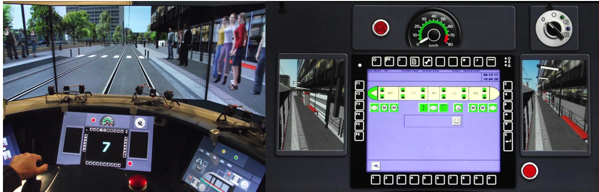
Fig. 10: Example of rear view display (right part) incoherent with the real direct outside view (left part)
