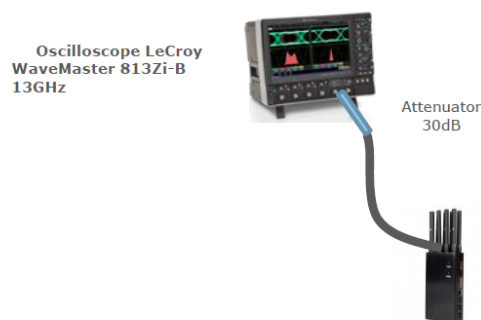
Fig. 1 Characterization of the signals produced by jammers accessible to general public
