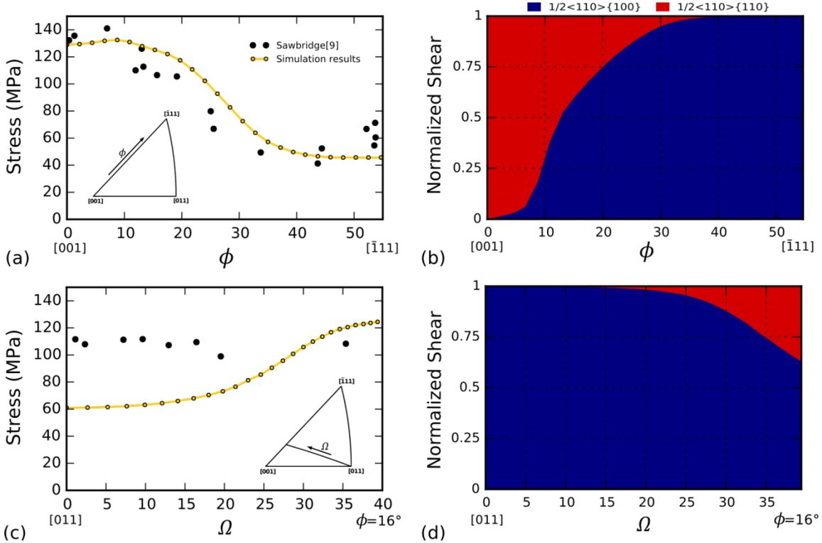
Figure 4: Stress anisotropy. (a)-(c) flow stress at 2% strain versus  $\phi$  and  $\Omega$  orientations. (b)-(d) Computed normalized plastic shear contribution for each slip mode ( $\gamma^{\{100\}}/\gamma_{tot}$  in blue and  $\gamma^{\{110\}}/\gamma_{tot}$  in red) versus  $\phi$  and  $\Omega$  orientations.
