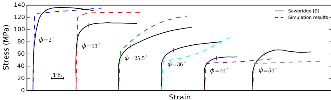
Figure 2: Stress-strain of 1600 K  $\text{UO}_2$  single crystal compression tests. CPFEM (dashed line) is compared to experimental compression tests (full line) [9]. Computed data are shown using the engineering stress definition.
