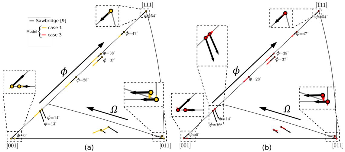
Figure 3: Lattice rotations in  $\text{UO}_2$  single crystal compression after 2% strain. Experimental lattice rotations (in black) versus computed rotations using the CPFE approach including (a) case 1 (in yellow) and (b) case 3 in red (model parametrizations are detailed in table 3).
