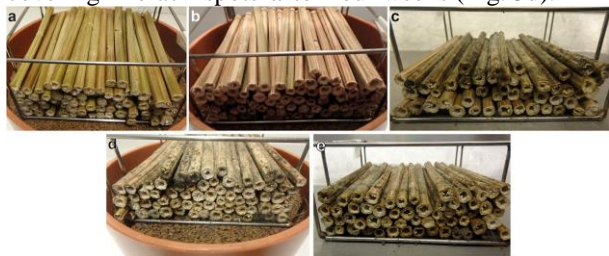
Fig. 3. Photographs of the hemp litter layers before and during the retting period: (a) before retting, after (b) 7, (c) 14, (d) 28 and (e) 42 days of retting.
