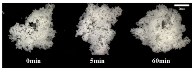
Fig. 3. Microstructure of the agglomerates of skim milk powder during drying at 110 °C as a function of the drying times (0, 5, or 60 min).
