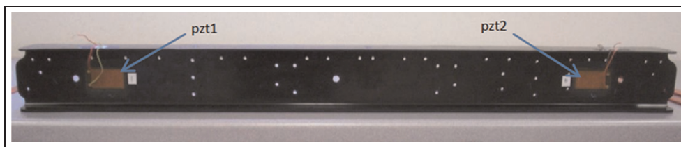
Figure 8. Instrumented composite stiffener, two DuraAct ® piezoelectric patches are bonded at the extremities (red zones).
