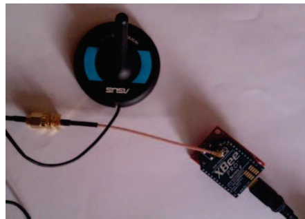
Figure 6: XBee receiver on the ground, linked to the ground station
