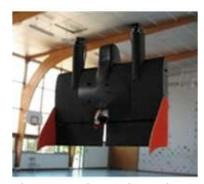
Fig.1 MAVion (Dimensions: 400mmx220mm) in hover configuration
