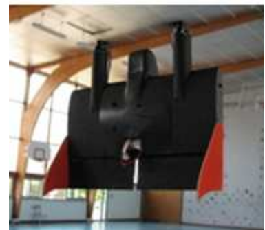
Fig.1 MAVion (Dimensions: 400mmx220mm) in hover configuration
