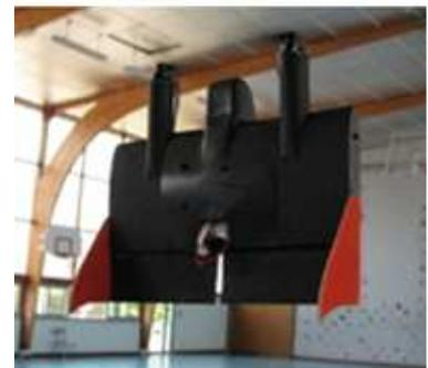
Fig.1 MAVion (Dimensions: 400mmx220mm) in hover configuration
