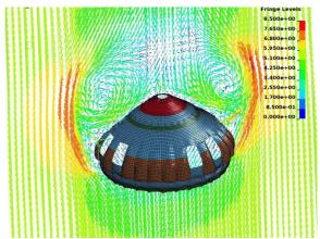
Figure 8. Fluid velocity vectors on a vertical section.
