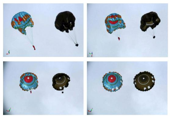
Figure 14. Real and computed profiles compared at different times during the opening.
