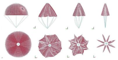
Figure 10. Parachute forming process using added mass.
