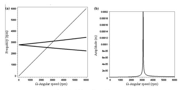
Fig. B. (a) Campbell diagram, (b) mass unbalance response.
