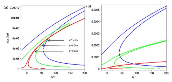
**Fig. 9.** Effect of variation in shaft diameter (a)  $\Omega = \omega_1$  (b)  $\Omega = \omega_2$ .
