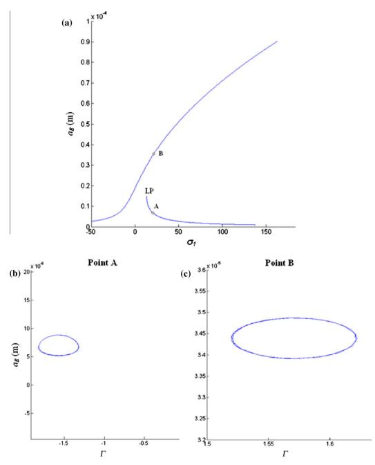
Fig. 3. Results obtained by continuation procedure using Matcont at  $\sigma_1$  = 20 for bifurcation diagram, (b) state plane at point A, (c) state plane at point B. 3.3. Case of  $\Omega = \omega_1$
