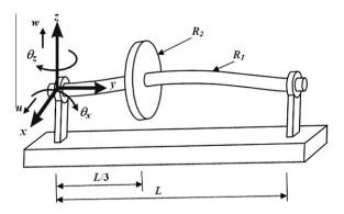
Fig. 1. Rotor with shaft and disk.
