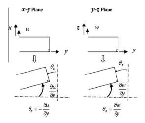
Fig. A. Transverse vibrations (beam in bending).
