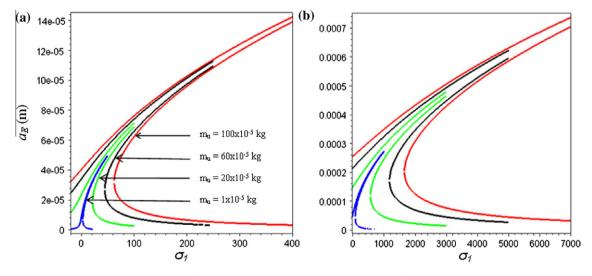
**Fig. 8.** Effect of variation in mass unbalance  $m_u$  (a)  $\Omega$  =  $\omega_1$  (b)  $\Omega$  =  $\omega_2$ .
