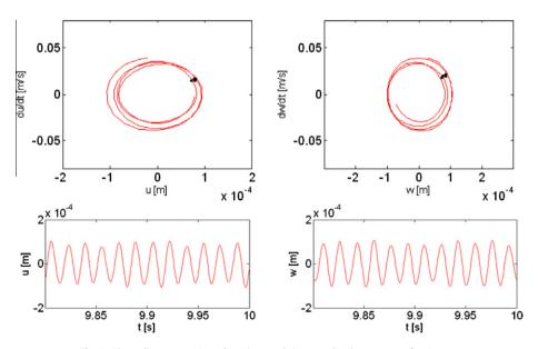
**Fig. 6.** Phase diagrams, poincaré sections and time amplitude responses for  $\Omega$  =  $\omega_2$ .
