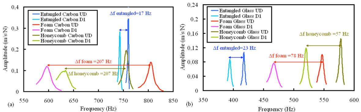
Fig. 7 Comparison of the frequency response functions estimated by sine-dwell testing for the undamaged case (UD) and damaged at 2 points (D1) for the 1<sup>st</sup> bending mode for (a) Point 11 for the three carbon sandwich beams and for (b) Point 21 for the three glass sandwich beams
