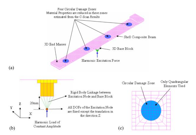
**Figure 5** Modeling methodology of damage in Samcef (a) Composite laminate beam model with end masses and base block showing the damaged zones and the excitation (b) Application of harmonic load at the excitation node situated 20 mm beneath the center of the base block (c) Close-up of the mesh around the position of damage where the material properties shall be reduced to simulate the damaged case
