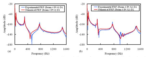
**Figure 10** Comparison of experimental/numerical FRFs for Beam 4 impacted by clamping all four ends for the damaged states D1 and D2 for the measurement points 4 and 32 respectively
