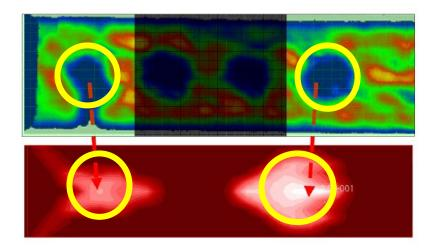
**Figure 9** Comparison between C-Scan results (top) and topology optimization (bottom) for the damage state D1 - The two middle impact points are blackened as they correspond to the damage state D2. Equivalent damage zone is identified using circle fitting matlab function and permits to estimate the radius of damage zone (yellow circles).
