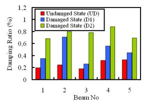
**Figure 8** Variation of damping ratios (%) estimated by Polymax for the five composite beams for 1st bending mode where 'UD' is the undamaged state, 'D1' is the damaged state at four points and 'D2' is the damaged state at eight points
