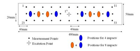
**Figure 2** Composite test-beams with location of damage, excitation and high spatial resolution for 33 measurement points
