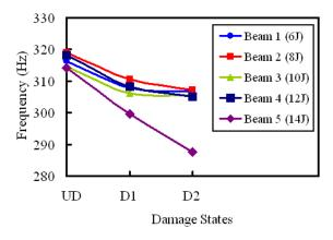
**Figure 7** Variation of damped natural frequencies with damage states for 2nd bending mode: UD is the undamaged state, D1 is the damaged state at four impact points and D2 is the damaged state at eight impact points
