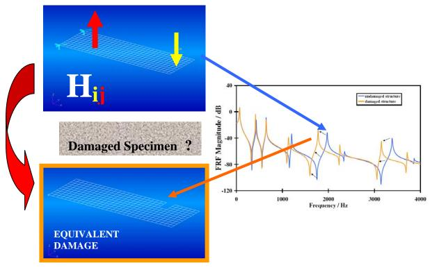
**Figure 3** Principle of damage localization using topology optimization method. The only a priori information is a baseline model (FEA) and the experimental modal data of the specimen under test [51]. The topology optimizer iterates until it minimizes the difference between experimental and baseline FRF and so on localize equivalent damages.
