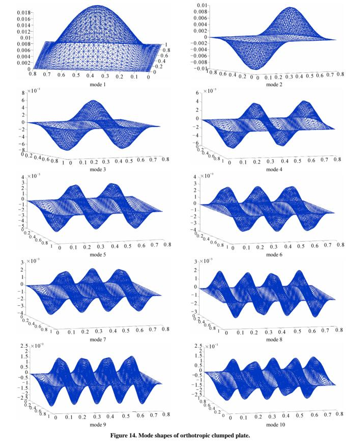
Figure 14. Mode shapes of orthotropic clumped plate.
