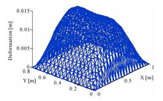
Figure 8. Deformation under a uniform distributed load.
