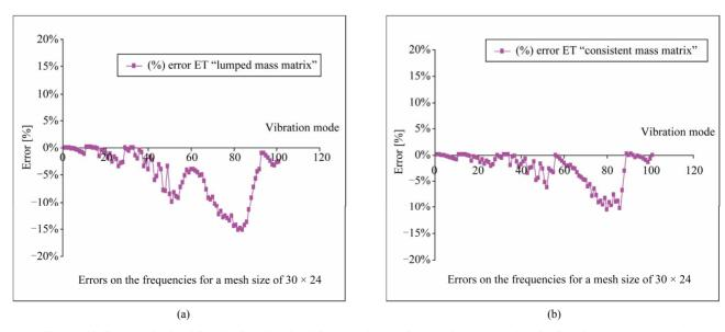
Figure 13. Errors obtained for the first hundred frequencies. (a) Lumped mass matrix; (b) Consistent mass matrix.
