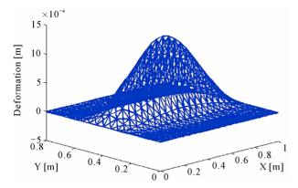
Figure 10. Deformed shape under a before concentred centred load.
