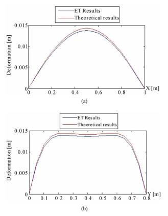
Figure 9. (a) Superposition of the median lines displacements along the "X" axis; (b) Superposition of the median lines displacements along the "Y" axis.
