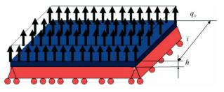
Figure 7. Simply supported plate submitted to uniform distributed load.
