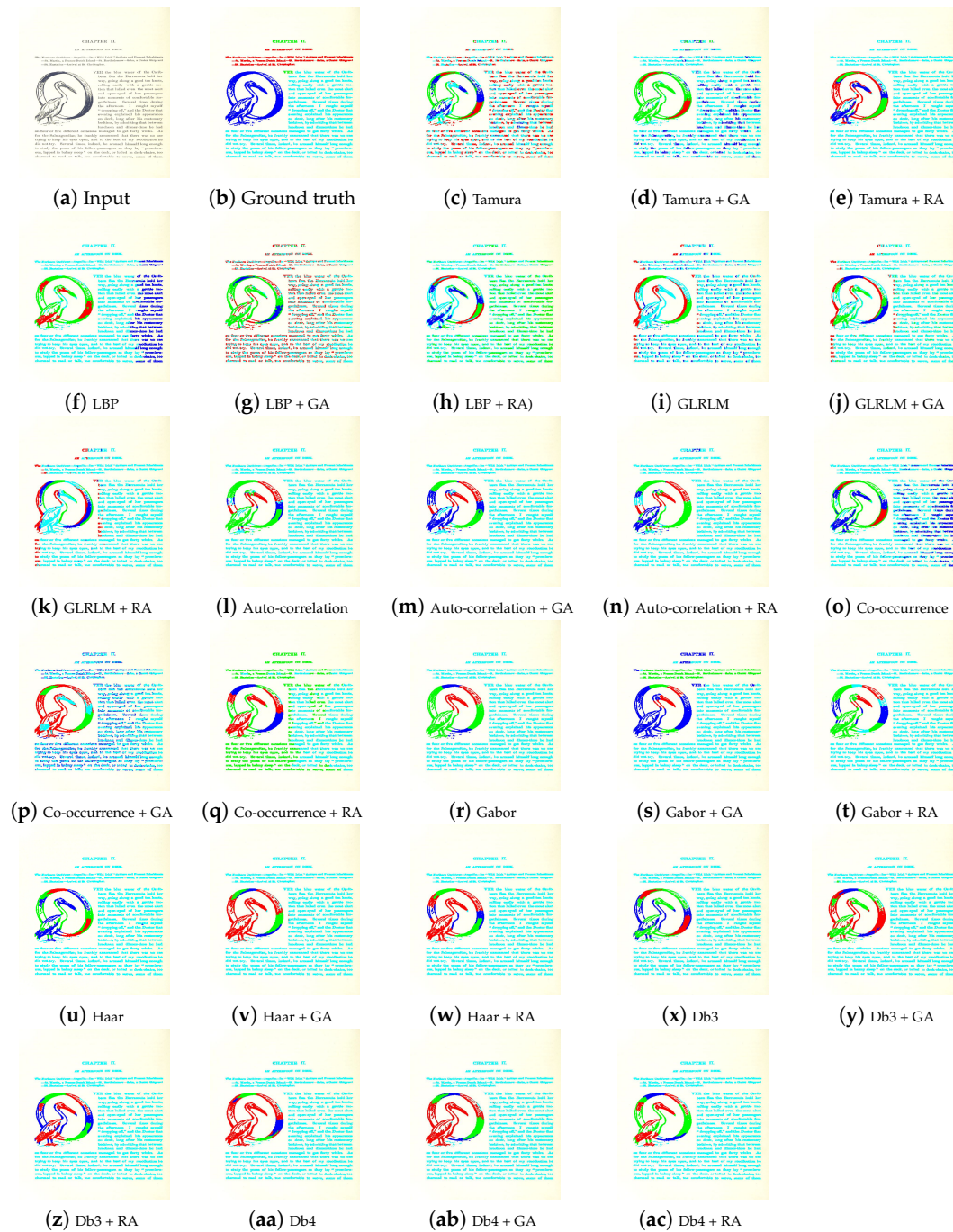
Figure 7. Qualitative results without and with using a feature selection algorithm on a historical document image of the “Three fonts and graphics” category from the testing dataset of the HBR2013 dataset . The number of class labels is equal to 4. Since the pixel-labeling task is unsupervised, the colors attributed to text or graphic clusters have been manually set to display the most correct matching. (a,b) illustrate the input image and its associated ground truth, respectively. The remaining figures depict the resulting pixel-labeling images. (c–e), (f–h), (i–k), (l–n), (o–q), (r–t), (u–w), (x–z) and (aa–ac) illustrate the resulting pixel-labeling images given by analyzing the full texture feature set (Tamura, LBP, GLRLM, auto-correlation, GLCM, Gabor, Haar, Db3 and Db4, respectively), the selected texture features by means of the GA and RA algorithms.
