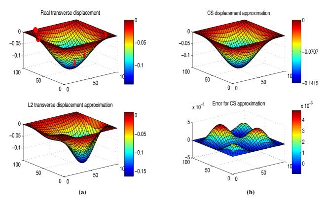
Fig. 6. First modeshape reconstruction of a SSSS plate. The sensors are in red (randomly chosen) on the 'continuous' modeshape (a) one can see the  $\ell_2$  inversion results on bottom. (b) We demonstrate the CS ability to reconstruct the modeshape, on bottom one can see the error versus continuous modeshape (maximum error of 5E-3).
