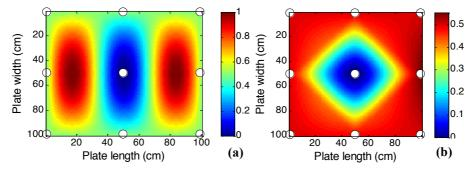
Fig. 1.: (3,1) mode of vibrating plate plus regular grid distribution of sensors in white circles (a) and The cubic interpolation which shows a spatial aliasing in mode shape reconstruction (b). A regular grid of 9 sensors permits only to reconstruct the (1,1).
