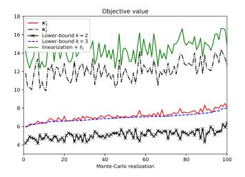
Fig. 3: Objective value and lower-bound given by our method (randomly driven filters, nonnegative case, T = 200). TABLE I: Final values of the objective function  $\mathcal{J}$  for various optimization methods (nonnegative case, T = 200).
