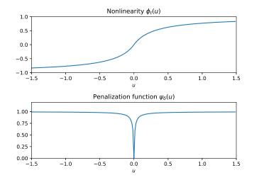
Fig. 1: Plot of the nonlinear saturation function  $\phi_t$  in (28) with  $\chi = 0.3$  and of the sparsity promoting function in (4) with  $\delta = 0.01$ .
