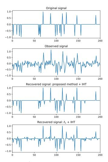
Fig. 6: Typical original signal  $\bar{\mathbf{x}}$ , observations d and recovered signal. These results have been obtained with IHT initialized either by our method or by using a linearized model and  $\ell_1$  penalty.
