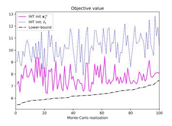
Fig. 5: Objective value for IHT with different initializations (randomly driven filters, real-valued case, T = 200). . TABLE II: Final values of the objective function  $\mathcal{J}$  for various optimization methods (real-valued case, T = 200).
