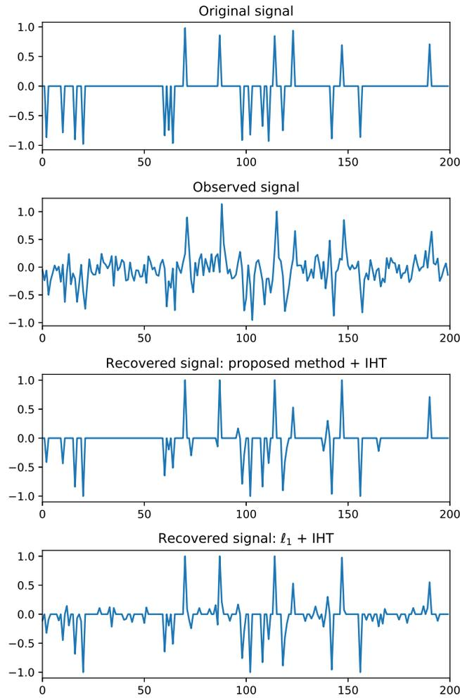
Fig. 6: Typical original signal  $\bar{x}$ , observations  $\mathbf{d}$  and recovered signal. These results have been obtained with IHT initialized either by our method or by using a linearized model and  $\ell_1$  penalty.
