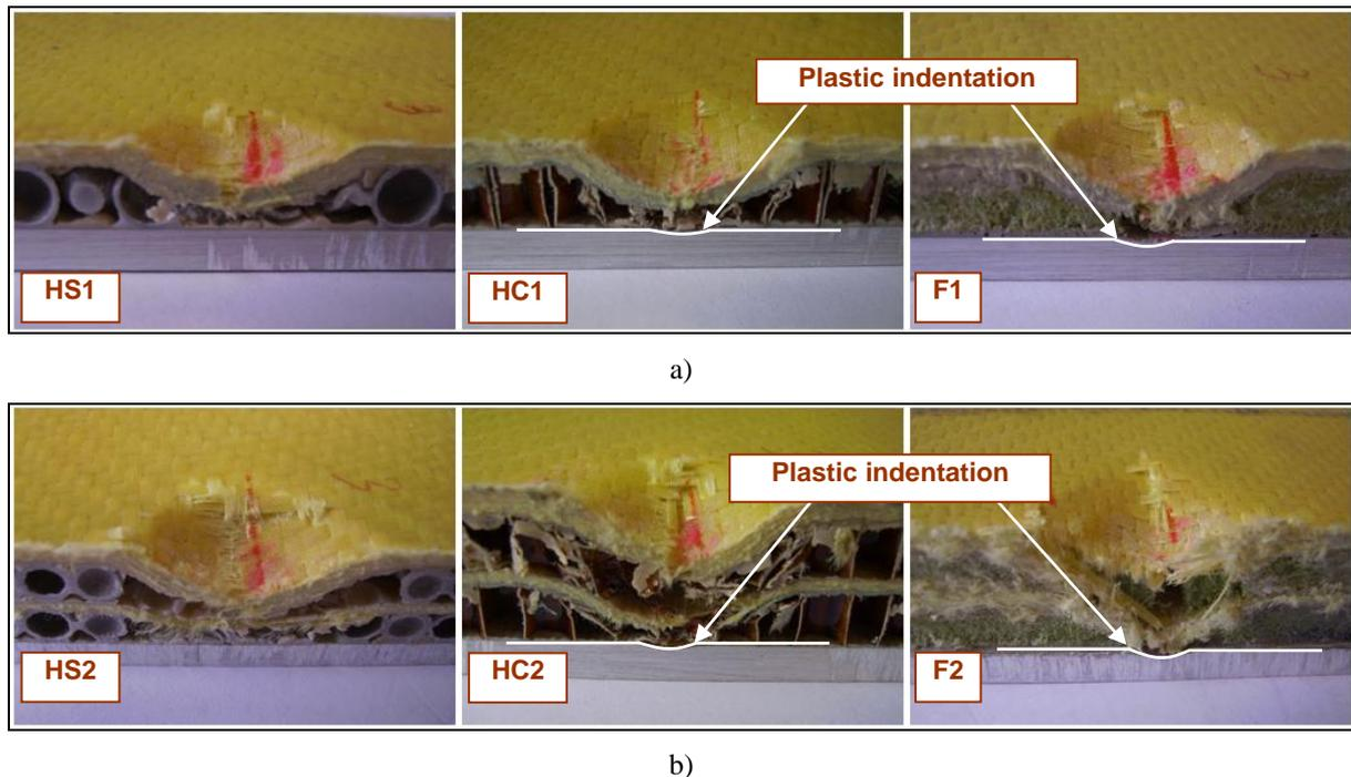
**Figure 4** : Cross-sections of impacted protective layers
