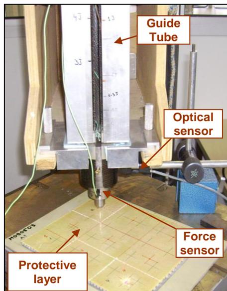
Figure 1 : Falling weight device
