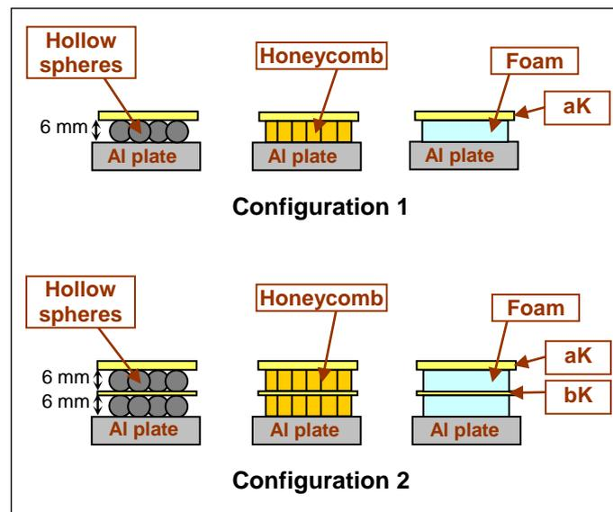
Figure 2 : Geometry and material configuration of protective layers
