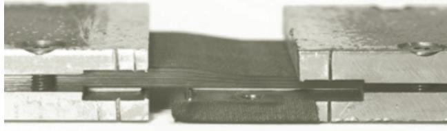
Fig. 4 Specimen clamped in the anti-buckling device
