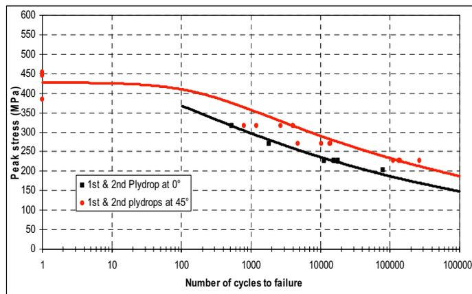
Fig. 12 Comparison of Stress/life curves for configuration with 1<sup>st</sup> & 2<sup>nd</sup> ply drops at 0° (v2) and at 45° (v5)
