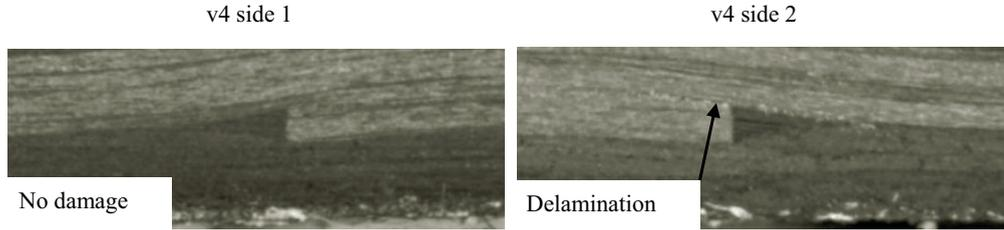
Fig. 8. Delamination at 2<sup>nd</sup> ply-drop of v4 tested at 50%, interrupted at 8000 cycles
