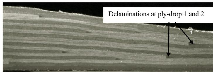
Fig. 7. Side 2 of v2 configuration tested at 50% and stopped at 10000 cycles with delaminations around ply-drop 1 and 2
