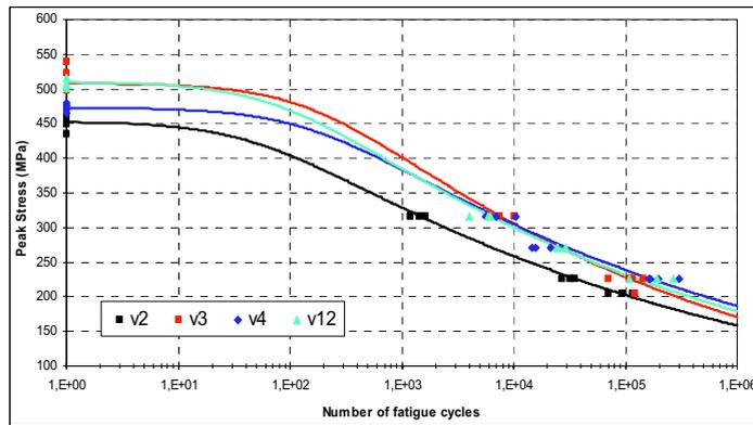
Fig.11 Stress/life curves for configurations with 1<sup>st</sup> & 2<sup>nd</sup> ply drops at 0°
