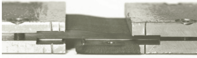
Fig. 4 Specimen clamped in the anti-buckling device
