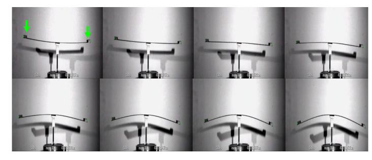
Fig 3: Oberst beam experimental set-up for the free-free beam excited at its centre. Half-period of the first mode is visualized from several successive frames. Virtual sensors are visualized with a small green dot; displacement is measured in Y direction (green arrows).
