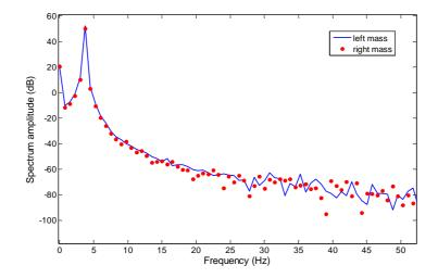
Fig 5: Frequency contents of the virtual sensors which highlight the expected harmonic mode of the beam at 3.8Hz.
