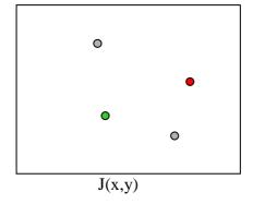
Fig 1: Optical flow principle. Pixel motion from image I to image J is estimated solving the pixel correspondence problem: given a pixel in I, look for nearby pixels of the same color in J. Two key assumptions are needed: color constancy (a point in I looks the same in J) and small motion (points do not move very far).
