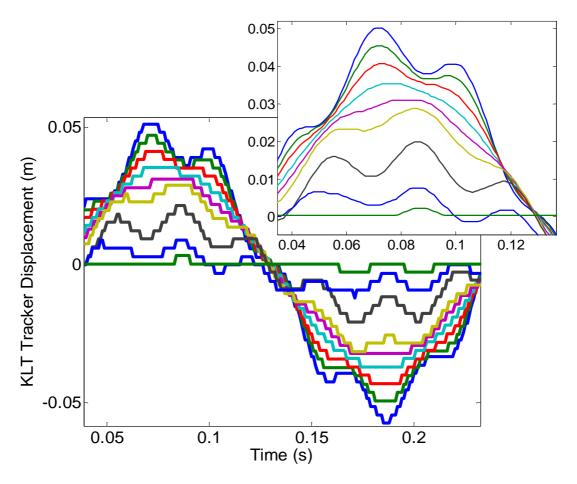
Fig 8: Experimental displacements measured on virtual sensors 1 to 9 sampled at FPS. The zoom on the enhanced displacement signaks shows the effect of the moving average function on the temporal signal. This pre-processing aims at obtaining smooth FRFs for better modal parameter estimation.
