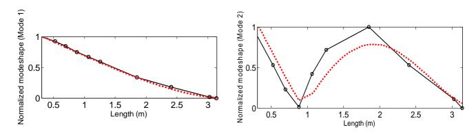
Fig 12: Two first mode shapes extracted using KLT on experimental data in black continuous line: The global content of these modes is very close to the two first mode computed using CATIA (red dotted line). Mode 1 is on top of the figure, mode 2 on bottom. The mode shape are normalized in order to be compared to FE modal analysis.
