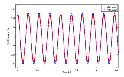
Fig 4: Validation of the algorithm using two virtual sensors on the left (blue line) and right mass (red dot line). The displacement (Y) is measured as a function of time. This displacements have an harmonic form according to the excitation frequency in this experiment close to the resonant frequency which appears at 3.8Hz (period of 0.26s).
