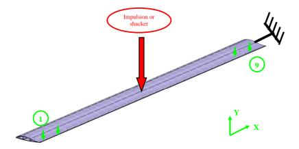
Fig 6: Helicopter blade example: KLT trackers are used to follow 9 targets in bending (Y displacement). The targets are numbered from 1 to 9, the blade is excited at its center.
