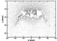
Figure 4 – Instantaneous velocity fields of the spray (left) and the gas phase (right) 4 ms after the start of injection for a single-hole injector
