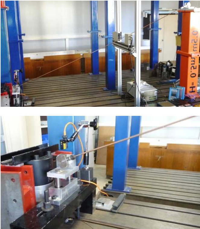
Figure 2: Experimental set-up: global view and detail of the excitation system.
