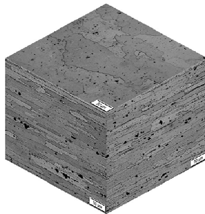
Fig. 1 - Optical microscopic 3D views of the AA 7175T7351 substrate after degreasing and metallographic attack.
