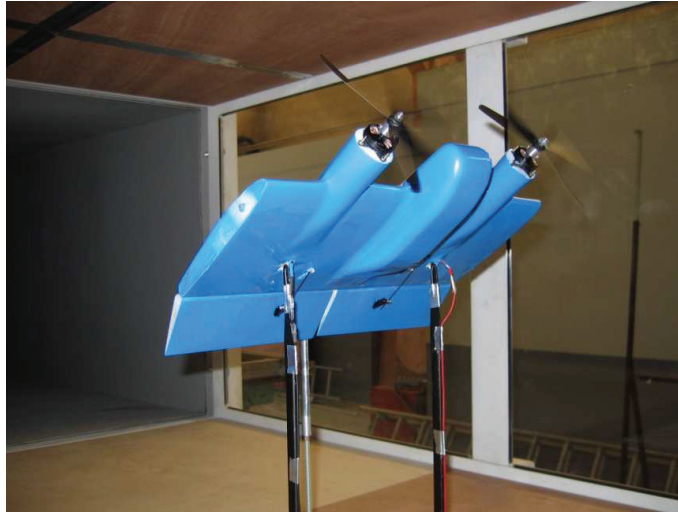
Figure 1: The MAVion, a convertible MAV developed in ISAE
