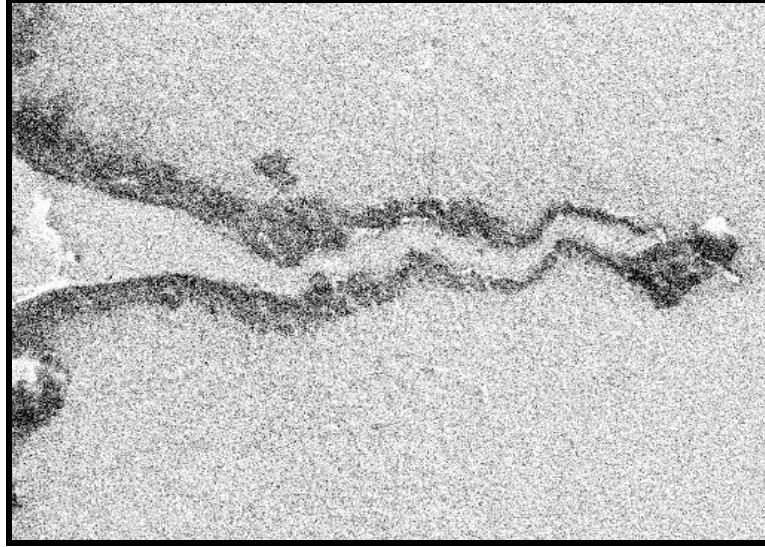
Figure 5 X-ray element map of oxygen of affected zone near crack edge
