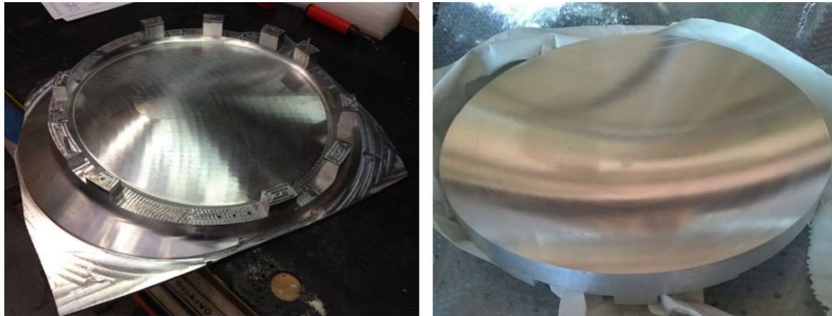
Figure 10. (a) The rear of the TD primary mirror being milled in the University of Milano Bicocca. (b) The front of the TD secondary mirror before polishing.
