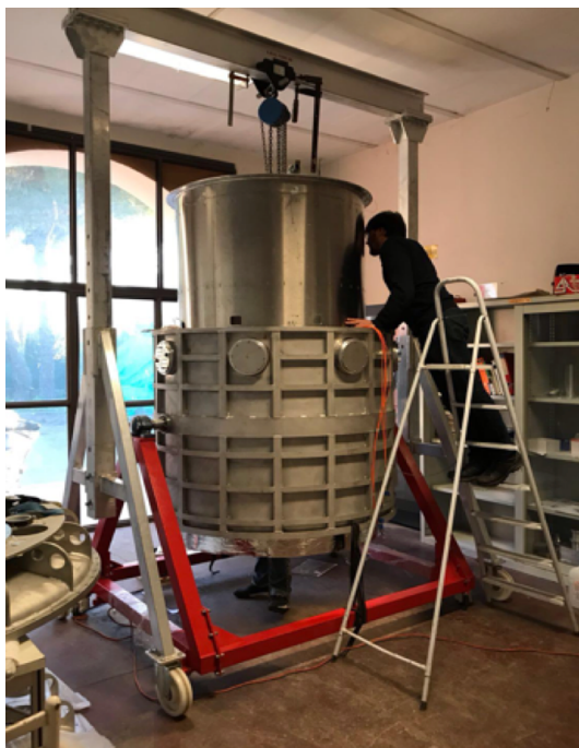
Figure 3: 40 K shield mounting in cryostat
