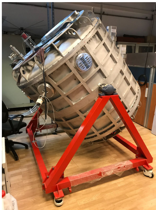
Figure 4: Closed cryostat under test
