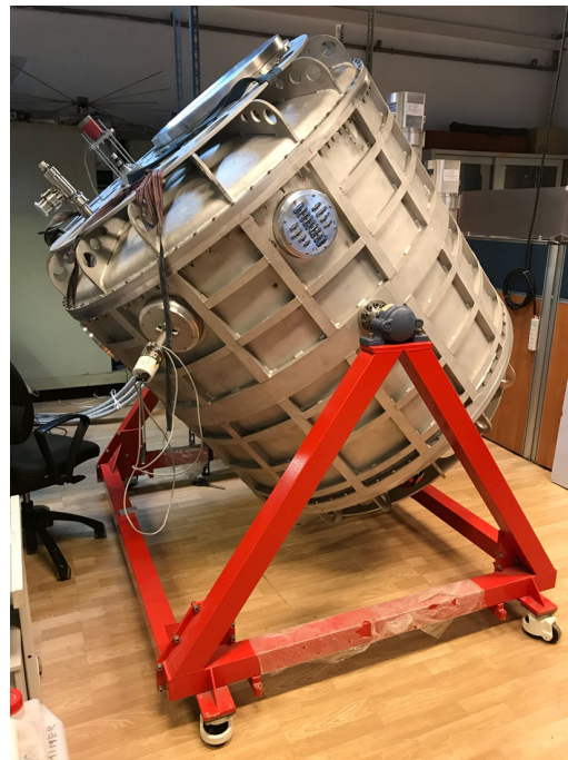
Figure 4: Closed cryostat under test
