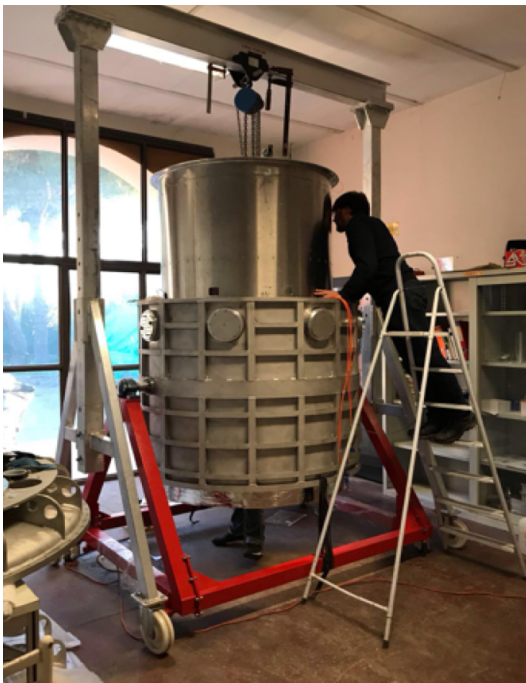
Figure 3: 40 K shield mounting in cryostat
