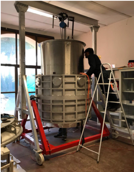
Figure 3: 40 K shield mounting in cryostat
