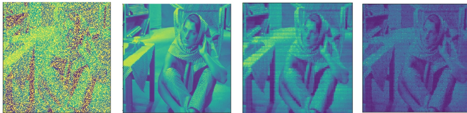
Figure 5: inpainting results from left to right: image with 50% of missing pixels, real image, Nonnegative OTLsingle , Unconstrained OTLsingle
