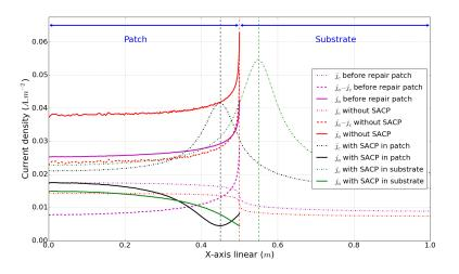
Figure 19: Situation 2 - Current densities along steel reinforcement  $(A.m^{-2})$
