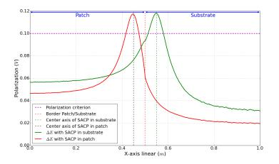
Figure 11: Situation 1 - Depolarisation values obtained with SACP embedded in the patch or in the substrate and criterion of efficiency for ICCP [39] (in dotted line)
