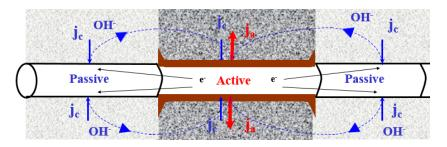
Figure 5: Situation 2 - Before patch repair
