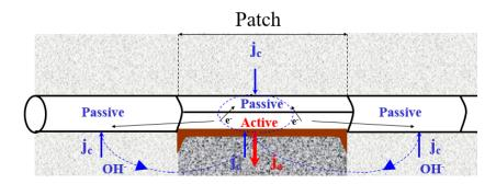
Figure 6: Situation 2 - After patch repair
