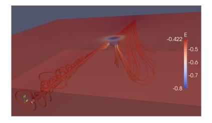
Figure 22: Situation 2 - 3D potential and current lines with a resistivity at 1000  $\Omega$ .m (V vs. SCE)
