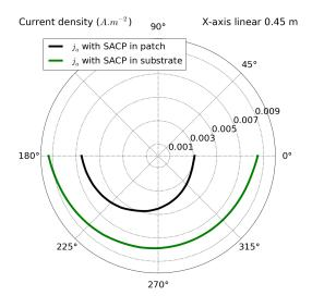
Figure 20: Situation 2 - Current distribution around the steel reinforcement depending on the angle  $(A.m^{-2})$
