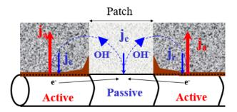
Figure 3: Situation 1 - Macrocell after patch repair
