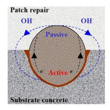
Figure 1: Illustration of macrocell corrosion around the steel
