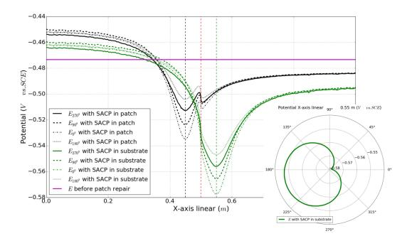
Figure 12: Situation 1 - Potential distributions along the steel reinforcement and around the steel reinforcement (bottom right) depending on the angle
