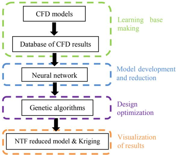
Fig. 1. Method of model reduction and optimization.
