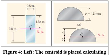
the half measure of each side of the rectangle (Beer et al., 2012, p. 247). Right: The centroid is placed using geometric formulae (p. 248).
