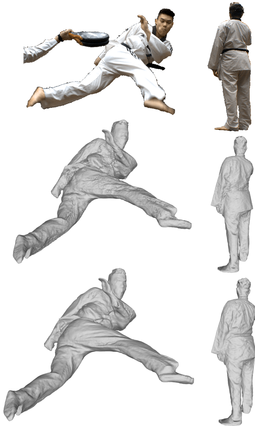
Fig. 7. ( Top ) input images, ( middle ) result with [22], ( bottom ) result with our method. Motion blur and low contrast are visible in the input images . Best viewed magnified.
